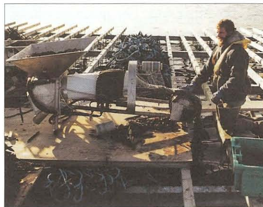
4. Binding mussels onto rope, using an Aguin roping machine.
