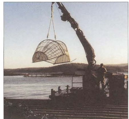
5. Hydraulic crane lifting a Spanish harvesting basket into position.
